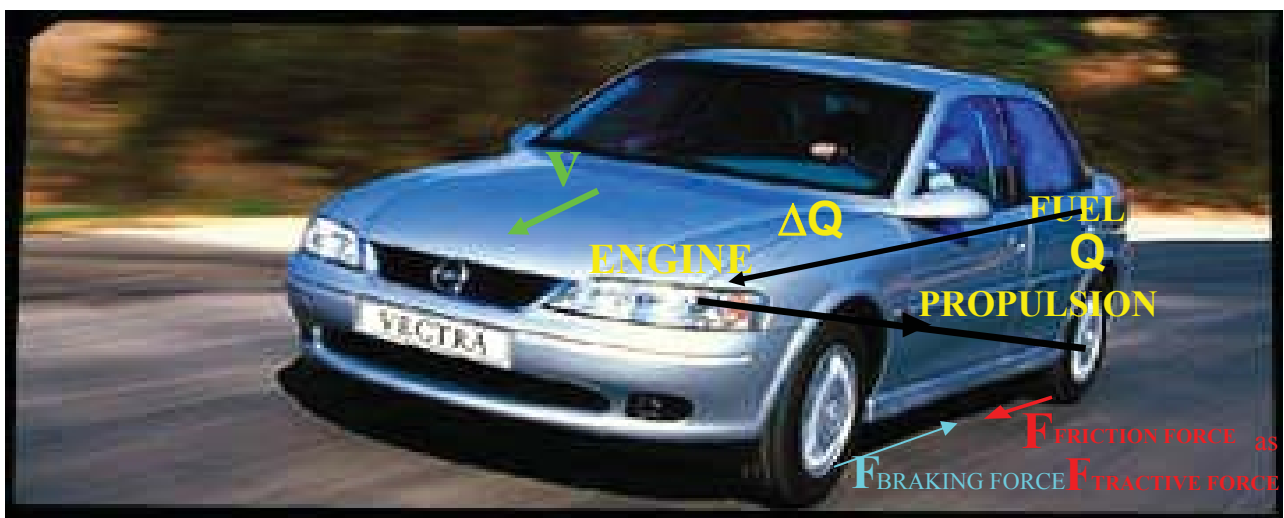
Fig.4. Rolling friction power as a vehicle driving power
