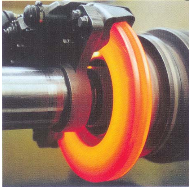
Fig. 3. A brake shoe – disc, tribological system
